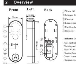
(1) White Fill Light (7) Button (2) Infrared Light (8) Microphone (9) Anti-Tamper Button (4) Loudspeaker (10) Terminals (5) Card Reading Area (1) Reset (2) TF Card Slot
