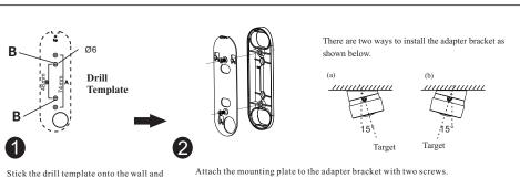
Stick the drill template onto the wall and then drill two holes according to the holes of the drill template marked with "**B**".
