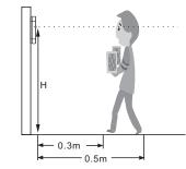
The recommended installation height (H) is 1.45m. It can be adjusted according to the actual scene.
